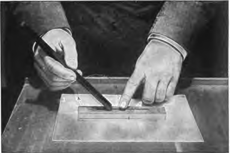
FIG. 9. REMAGNETIZING THE COMPASS-NEEDLE.
